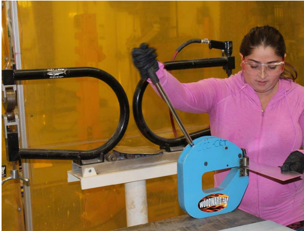
Kimberley Padilla, a native of Mora, measures metal on a metal shrinker stretcher machine in a recent class.
