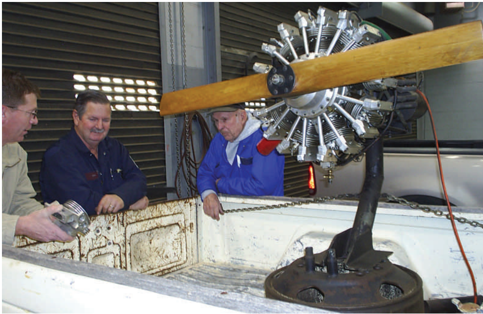
LCC Springer Satellite student Jimmy Caldwell examines one of the cylinder heads of a nine-cylinder radial engine with LCC Instructor Bill Jump and J.D. Schmidt, builder of the engine.
