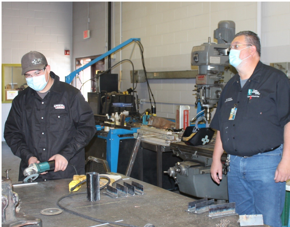
Left: Luna student Isaiah Dominquez grinds a 22.5 degree edge for a test plate as instructor Gene Martinez provides guidance.
