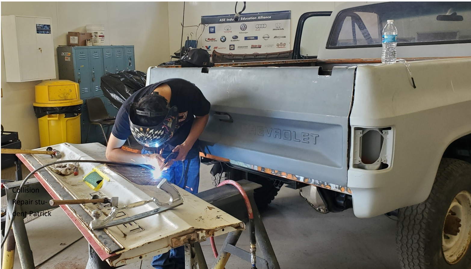
Luna collision repair student Patrick Antrillo welds a patch panel on a tailgate. Students in the collision repair program learn realistic hands-on training
