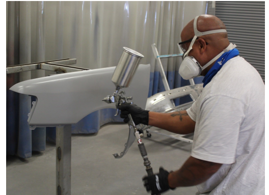
Above: Student Josh Vigil begins primer painting of a fender. Below: Student Joseph Sedillo prepares a tailgate for a body filler.
